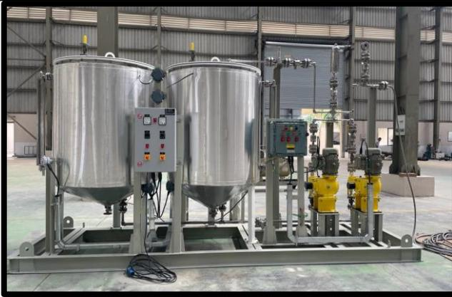
into the main product line. It mainly consists of additive storage tank, metering pump with flameproof Motor, Strainer, Pulsation Dampener Pressure Gauge, Non Return Valve, Bail valve, Back Pressure Valve to maintain the dosing Pressure, Level Transmitter, Base skid.
